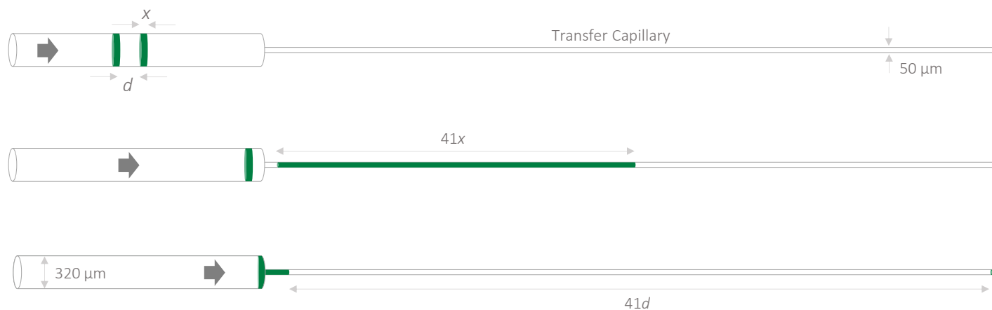
Fig 10. AES' IDTT (Inner Diameter Transfer Technology) patent. As the charge variant zones go from the 320 \mu\text{m} diameter icIEF capillary to the 50 \mu\text{m} diameter transfer capillary, the separation distance will increase by approximately 41 times, and therefore reduce the cross-contamination caused by molecular diffusion and the parabolic velocity flow profile. The pressure mobilization enables excellent consistency and speed while avoiding the chemical mobilization additives that can cause instabilities related to Joule heating and pH gradient disruption. The last peaks to elute will have the worst purity due to the extra-column effects influencing the preceding samples. Fortunately, pressure mobilization also supports reversed polarity to allow the acidic variants to elute first for a higher purity.
